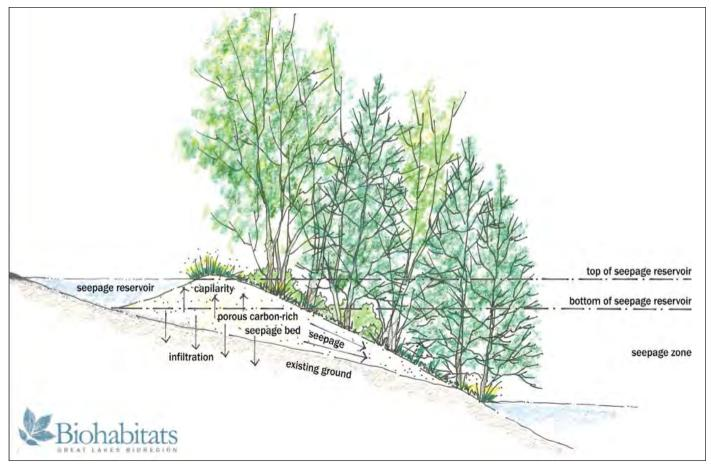
Figure 40. A typical cross section of a sand seepage berm design (Copyright Biohabitats Inc.).
